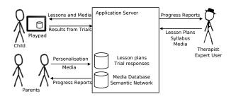
Figure 1: System Architecture
